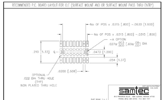
Figure 9: recommended footprint for the Samtec connector of the receiving board.
