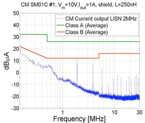
Figure 5: typical output common mode current.
