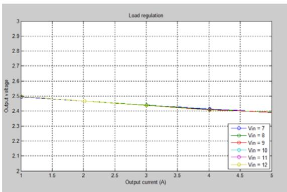
Figure 4: typical load regulation properties.
