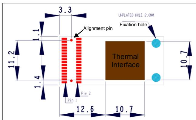
Figure 8: recommended footprint to be implemented on the receiving board.
