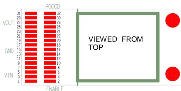
Figure 2: Top view and pin numbering of the power interface
