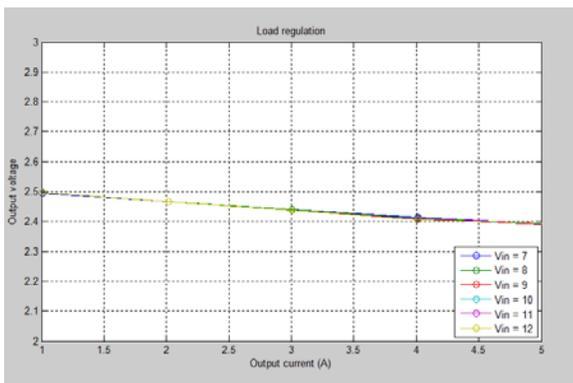
Figure 4: typical load regulation properties.
