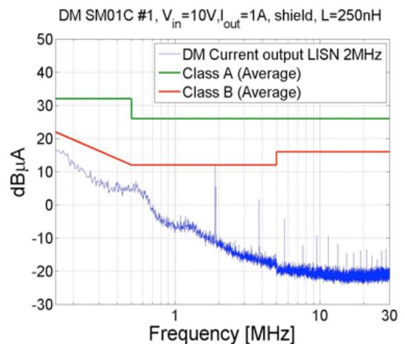
Figure 6: typical output differential mode current.
